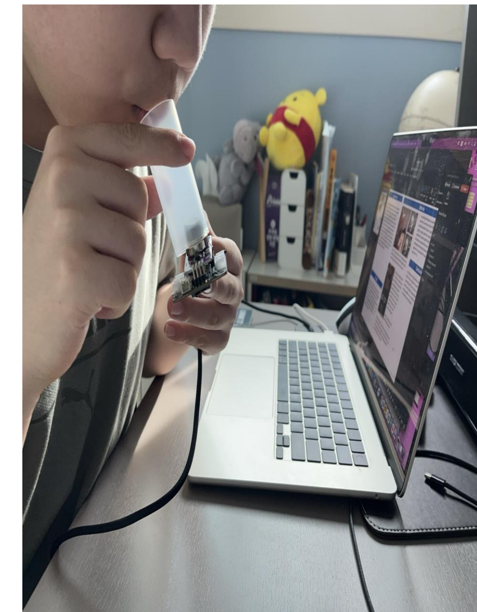
Figure 3: participant exhaling toward the VOC sensor through the mouthpiece
