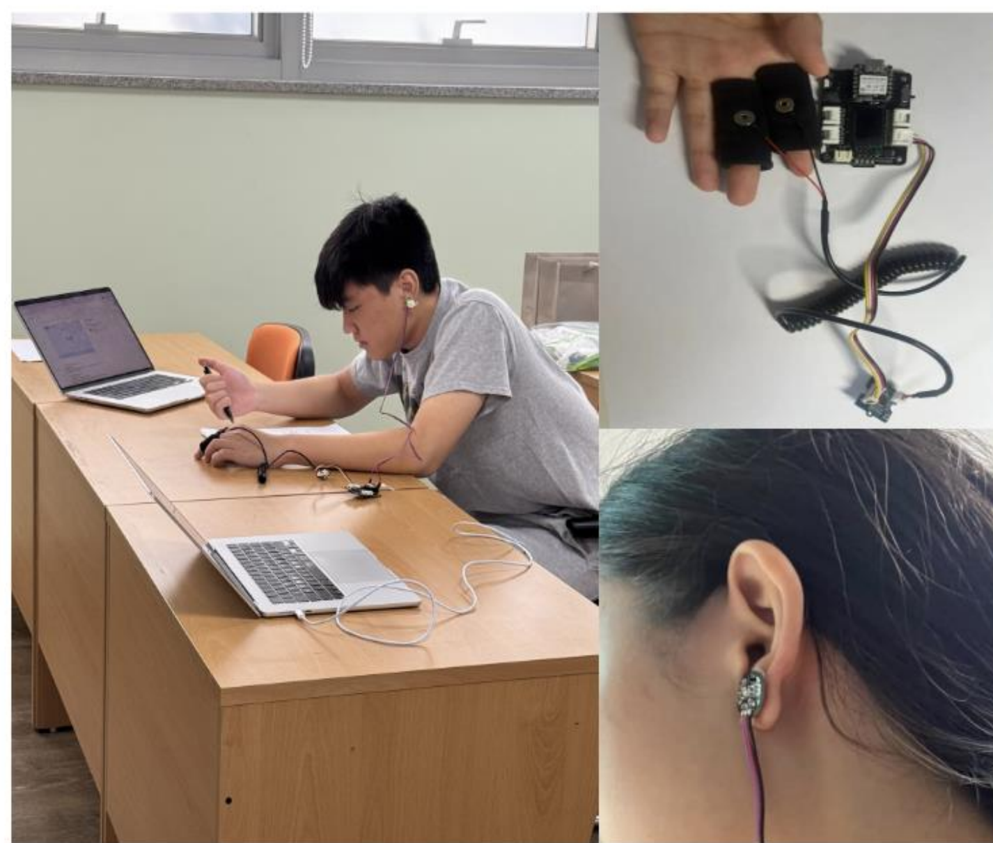
Fig 2. The participant wears a PPG sensor on the earlobe and GSR sensors on the index and middle fingers during the exam.
